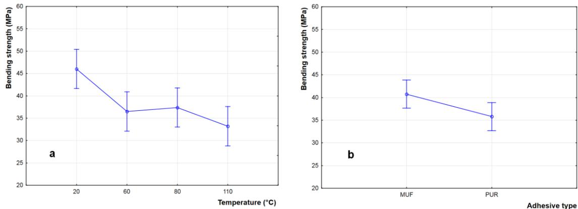
**Fig. 5.** Influence of (a) temperature and (b) adhesive type on bending strength
