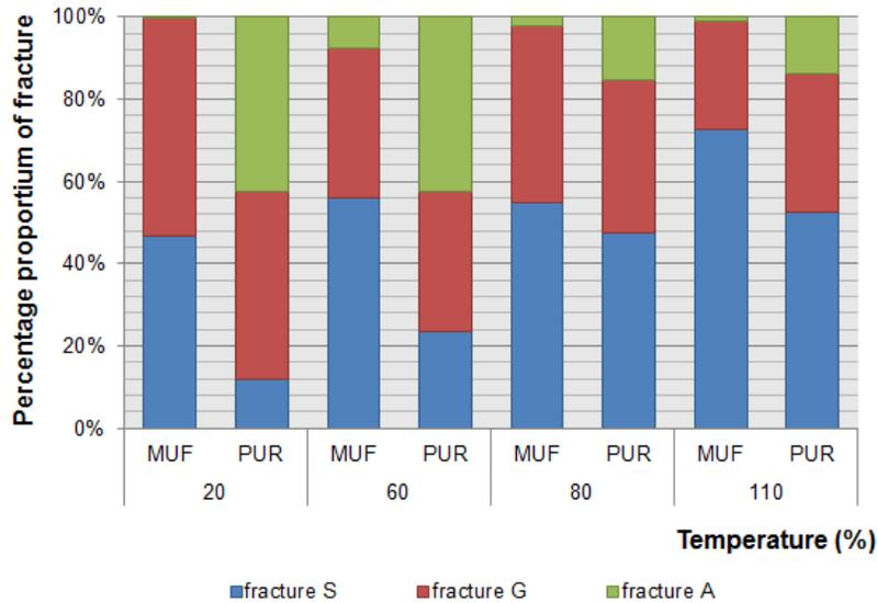
**Fig. 9.** Proportion of fracture types in finger joints
