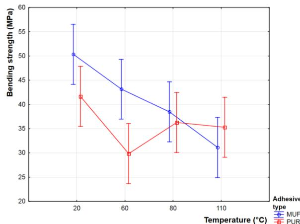
**Fig. 6.** Influence of temperature and adhesive type on bending strength
