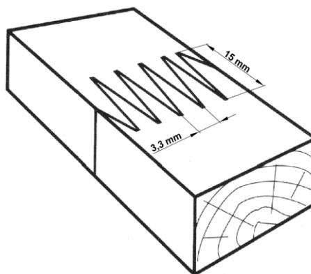
**Fig. 2.** Dimensions of finger joint
