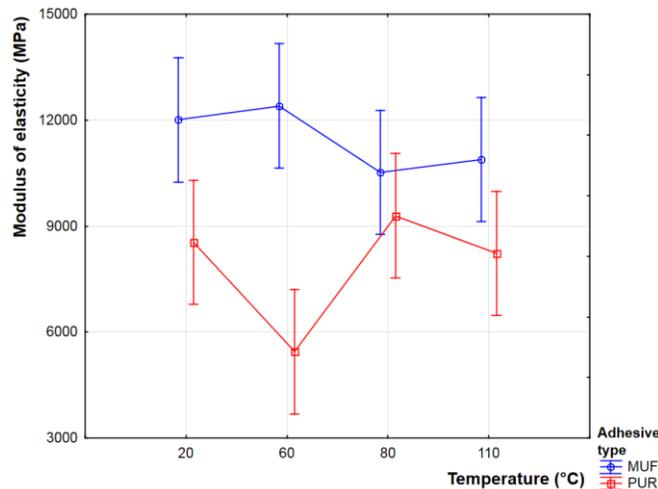
Fig. 8. Influence of temperature and adhesive type on modulus of elasticity
