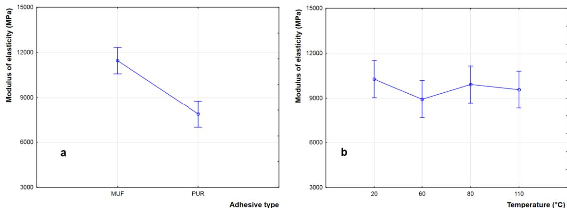
**Fig. 7.** Influence of (a) temperature and (b) adhesive type on modulus of elasticity
