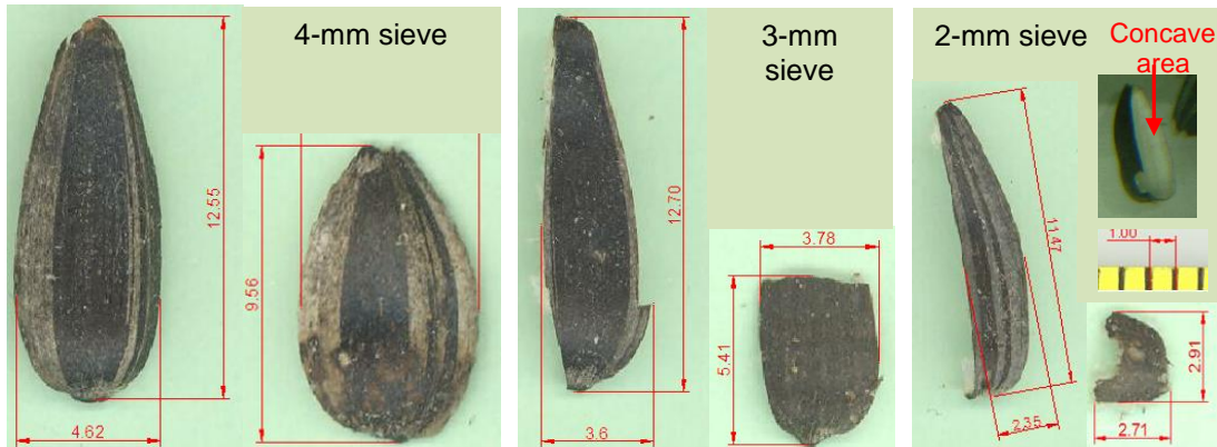
Fig. 2. Geometry and size of coarse particles measured in AutoCAD program, in mm
