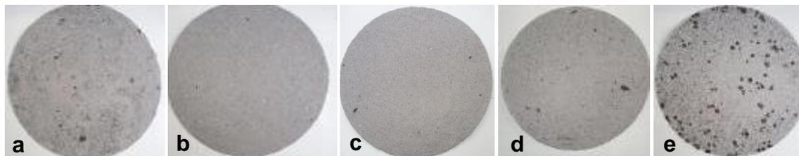
**Fig. 5.** The carbon fiber composite paper-sheets with different dispersants. (a) SCF without dispersant, (b) SCF treated with PS-80 (c) SCF treated with CPAM, (d) SCF treated with CTAB, and (e) SCF treated with SDS
