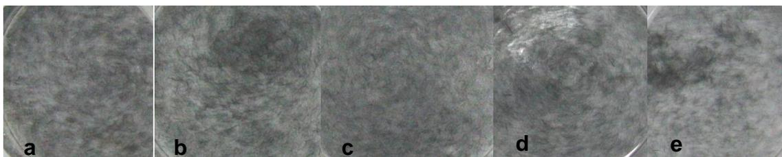
**Fig. 4.** Dispersants applied to SCF suspensions; (a) SCF without dispersant, (b) SCF treated with PS-80, (c) SCF treated with CPAM, (d) SCF treated with CTAB, and (e) SCF treated with SDS
