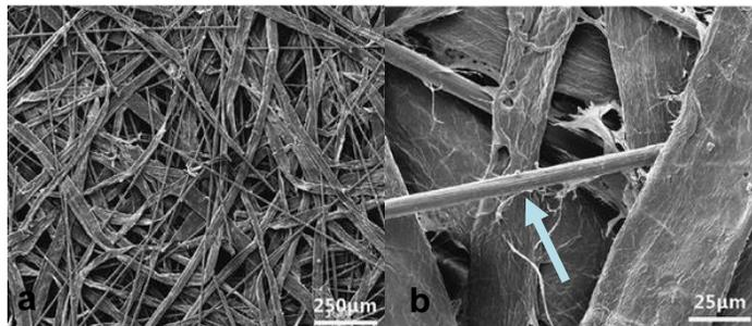
**Fig. 6.** SEM images of the SCF / PF composite papers (40 wt% of SCF)
