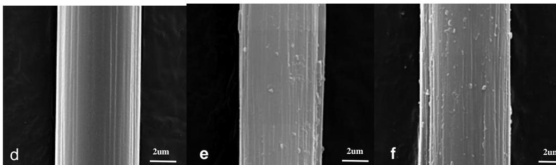
**Fig. 3.** SEM images of (d) SCF after liquid acid oxidation, (e) TMC-102 treatment, and (f) KH-550 treatment
