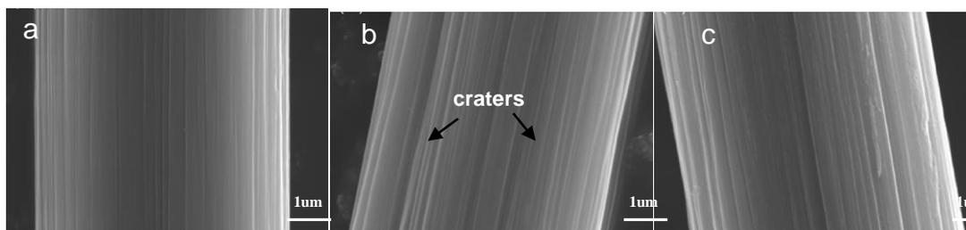
**Fig. 2.** SEM images of (a) untreated SCF, (b) SCF after isothermal holding at 400 °C for 1 h, and (c) SCF after H<sub>2</sub>SO<sub>4</sub>/KClO<sub>3</sub> treatment for 1.5h
