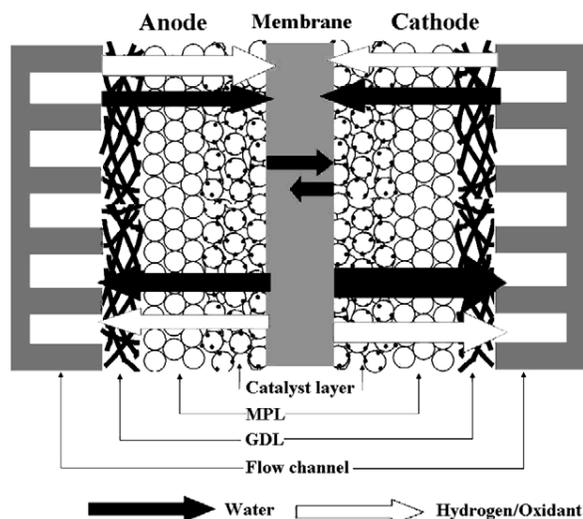
Fig. 1. Schematic diagram of a PEMFC
