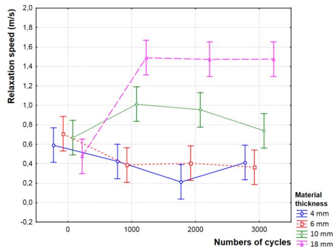
**Fig. 7.** Effect of numbers of cycles and material thickness on the relaxation speed for laminated wood. Data reported as mean ± SD
