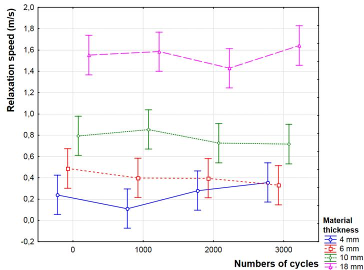
**Fig. 5.** Effect of numbers of cycles and thickness on the relaxation speed for native wood. Data reported as mean  $\pm$  SD
