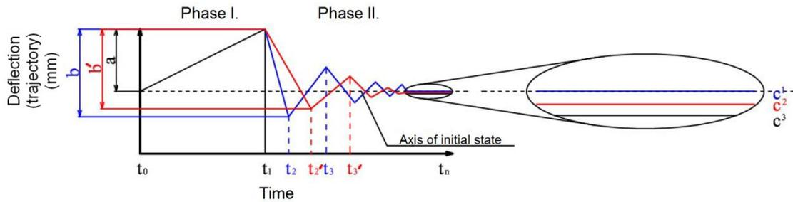
**Fig. 2.** Principle of shape deviation after cyclic loading (Phase I. – loading, Phase II. – releasing, a – deflection, b, b' – trajectories,  $t_0$  – initial state,  $t_1$  – time of unloading,  $t_2$ ,  $t_2'$ ,  $t_3$  and  $t_3'$  – times of relaxations and,  $c^1$ ,  $c^2$ , and  $c^3$  – final relaxed shapes)
