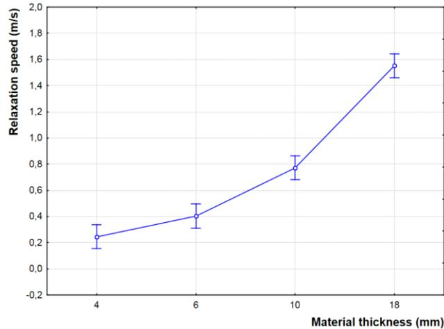
**Fig. 4.** Effect of material thickness on the relaxation speed for native wood. Data reported as mean  $\pm$  SD
