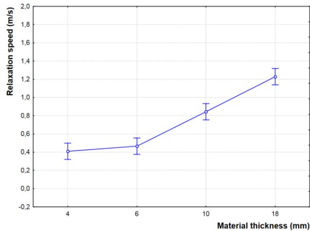
**Fig. 6.** Effect of material thickness on the relaxation speed for laminated wood. Data reported as mean ± SD
