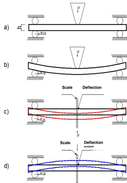
**Fig. 3.** Illustration of deflection for laminated wood: (a) before loading, (b) maximum load is applied, (c) releasing the maximum load, and (d) return of wood to original state
