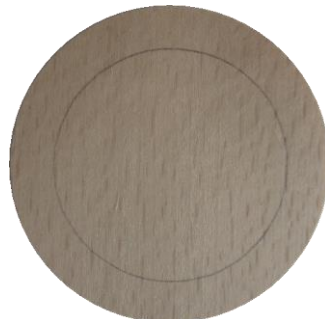
Fig. 1. Test piece with the drawn auxiliary circle
