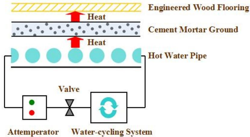
**Fig. 3.** The process of heat transfer
