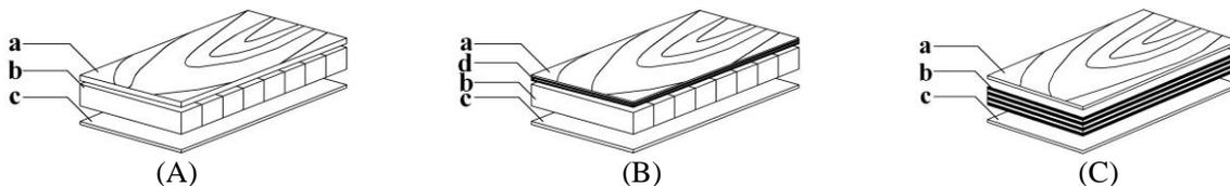
**Fig. 1.** Three types of structure (A), (B), and (C) of engineered wood flooring: (a) decorative face (upper) veneer, (b) core board, (c) back (lower) board, and (d) plywood
