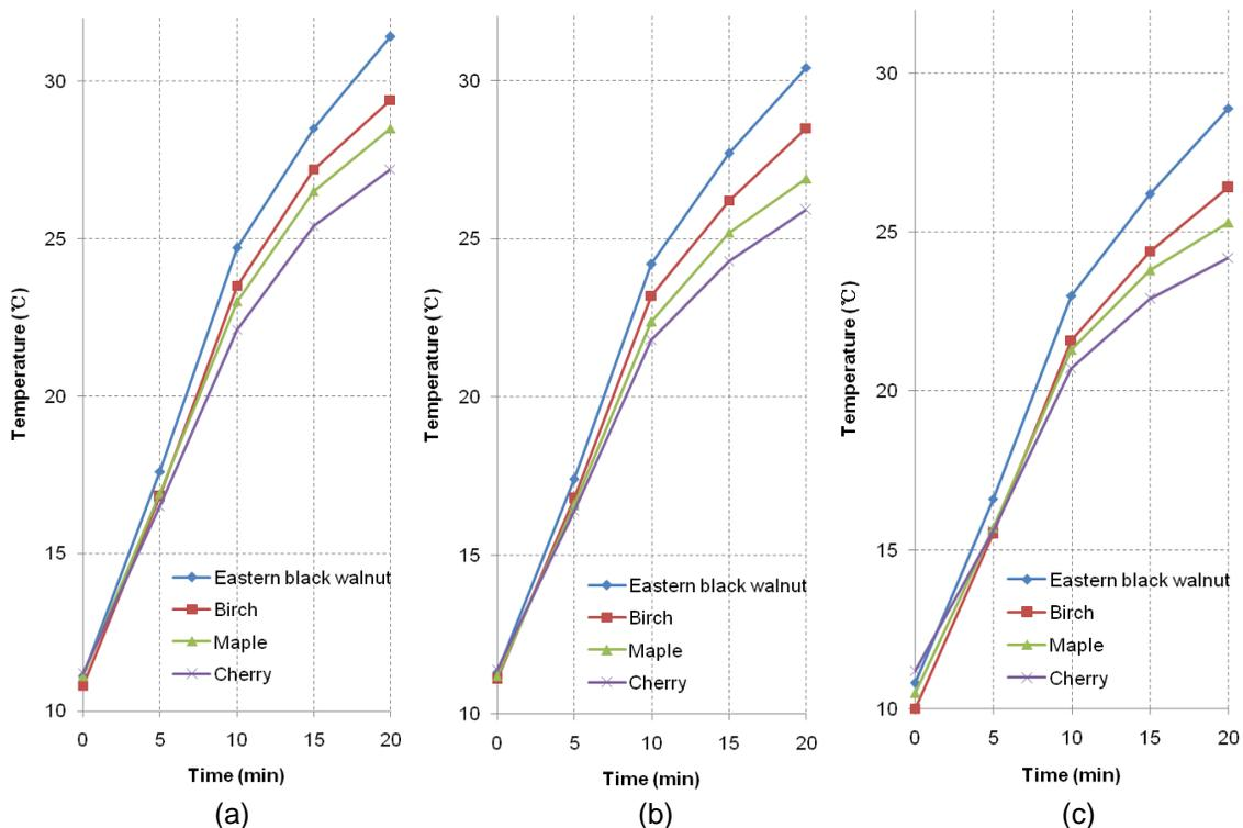
**Fig. 4.** The upper surface temperature trends for engineered wood floorings that were decorated with four different veneers: eastern black walnut, birch, maple, and cherry. (a) structure A, (b) structure B, and (c) structure C
