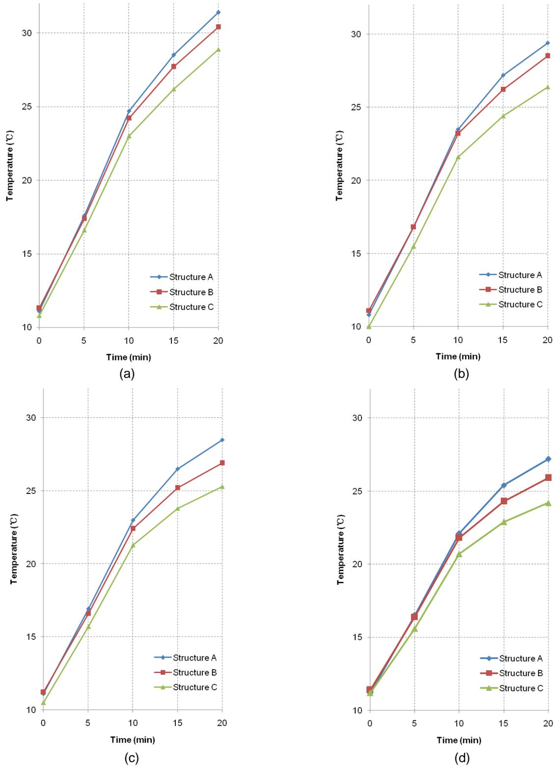
**Fig. 5.** The temperature uptrend of different engineered wood flooring structures: (a) Eastern black walnut, (b) Birch, (c) Maple, and (d) Cherry
