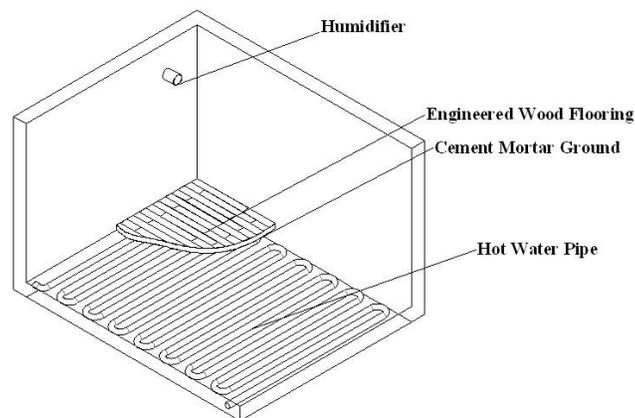
**Fig. 2.** The testing environment
