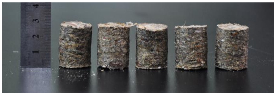
Fig. 4. Briquettes made under 60 MPa in the CS content of 50% at moisture content of 9%
