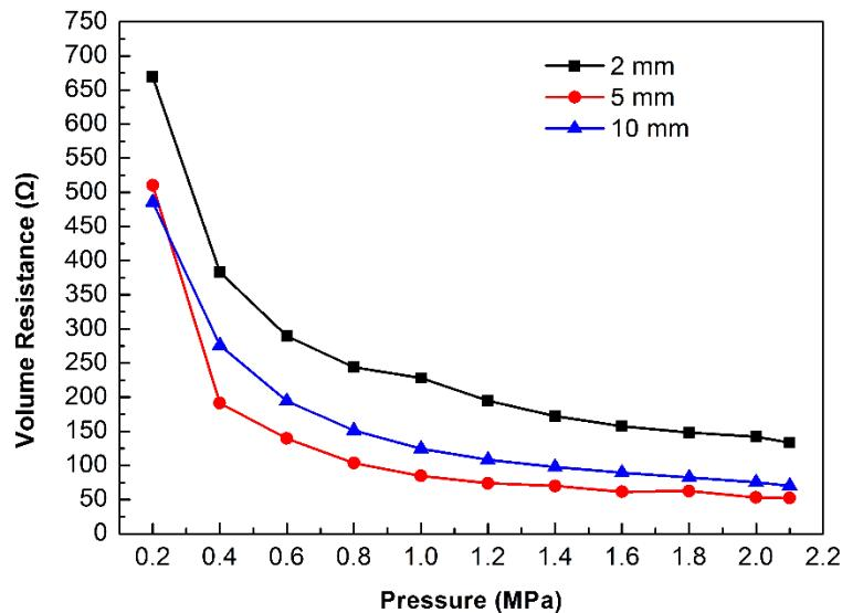
**Fig. 6.** The volume resistance of fiberboards under external pressure
