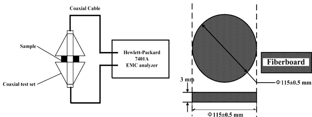
**Fig. 3.** The setup and specimen sizing for the electromagnetic shielding effectiveness test
