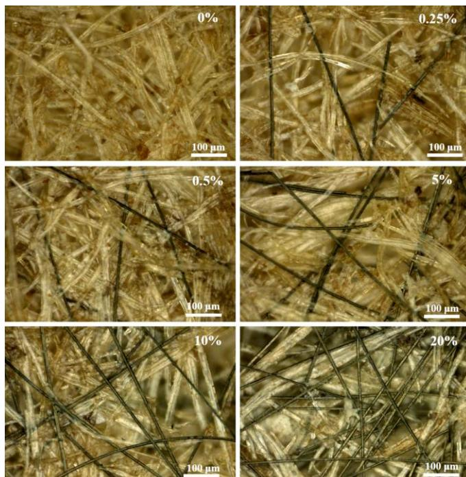
**Fig. 4.** CF distribution in the plane of fiberboards. The black fibers are CFs, and the brown fibers are wood fibers
