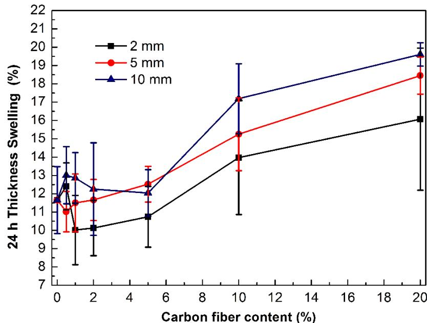
**Fig. 11.** Thickness swelling of fiberboards with different lengths and contents of CF
