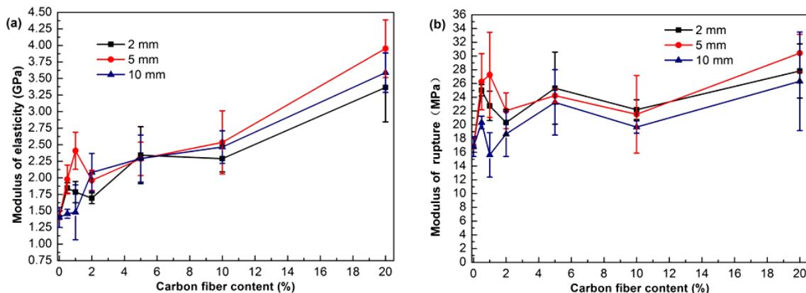
**Fig. 10.** (a) MOE and (b) MOR of fiberboards with various CF lengths and contents
