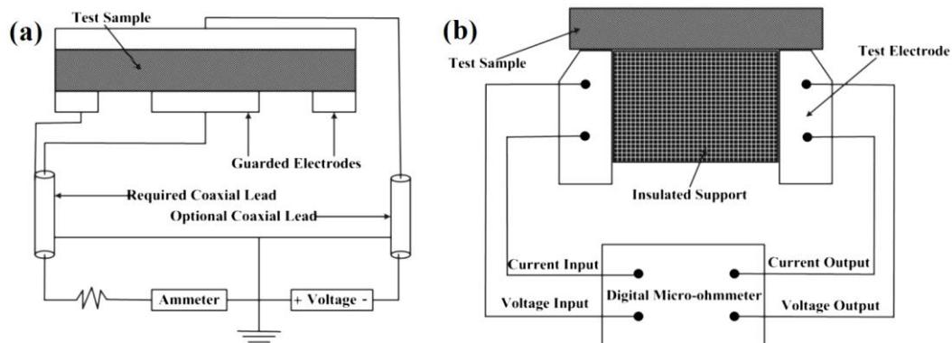
**Fig. 2.** Setup for measuring the (a) insulation resistance and (b) DC low-resistance
