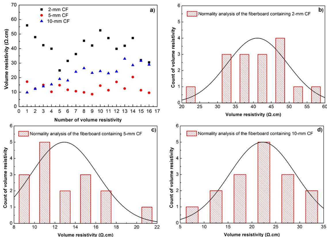
**Fig. 7.** Normality analysis for the volume resistivity of the fiberboards: a) Volume resistivity of the fiberboards; b) Normality analysis of the fiberboard containing 2-mm CF; c) Normality analysis of the fiberboard containing 5-mm CF; and d) Normality analysis of the fiberboard containing 10-mm CF
