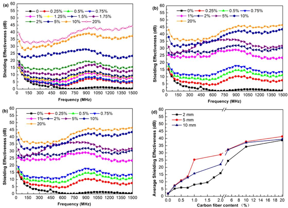
**Fig. 9.** SE of fiberboards with various CF lengths and contents: (a) CF length of 2 mm; (b) CF length of 5 mm; (c) CF length of 10 mm; and (d) mean SE of the fiberboards
