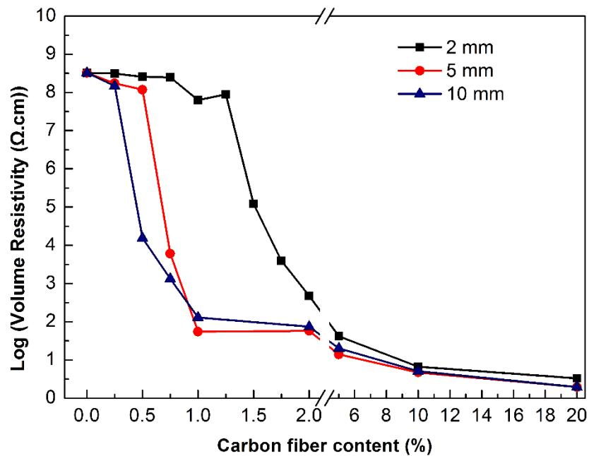
**Fig. 8.** The effect of CF length and content on the volume resistivity of fiberboards
