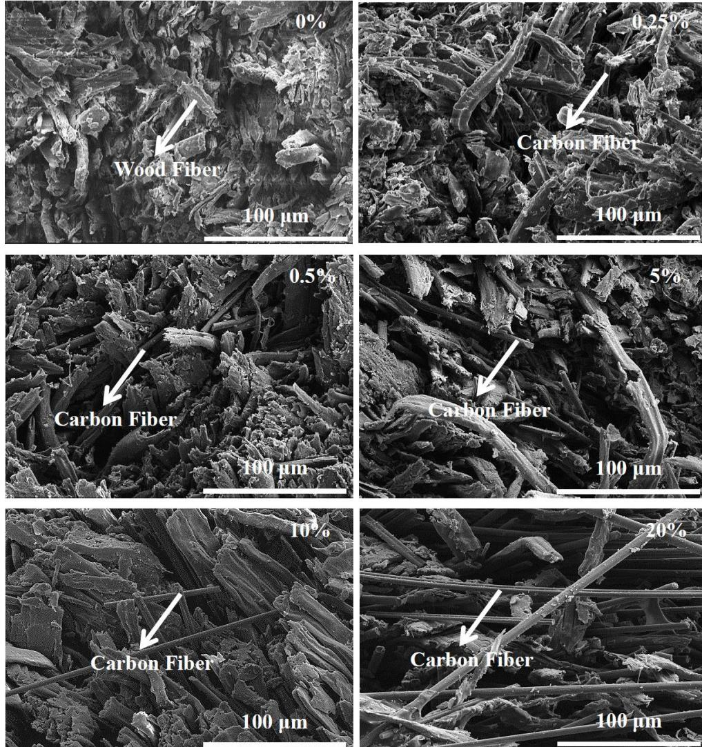
**Fig. 5.** CF distribution in the cross-section of the fiberboards
