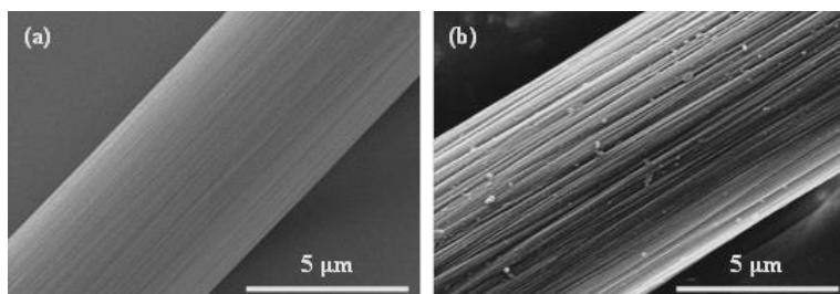
**Fig. 1.** The CF surface morphology (a) before and (b) after surface pretreatment
