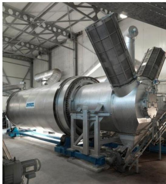
**Fig. 8a.** Rotary drum reactor (Thamer 2013)
