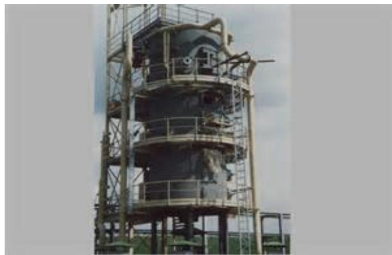
**Fig. 10a.** Multiple hearth furnace ([fgcgroupllc.com](http://fgcgroupllc.com))
