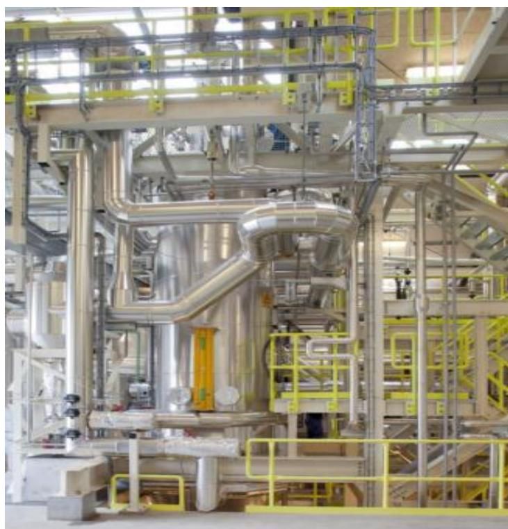
**Fig. 13a.** Moving bed reactor (Thamer 2013)
