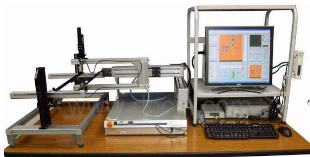
Fig. 6. The ACU C-scan imaging system used in this work
