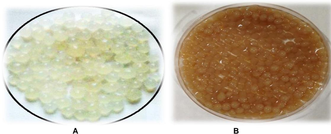
**Fig. 2.** Ca-alginate beads: (A) normal Ca-alginate beads; (B) Ca-alginate beads with immobilized laccase
