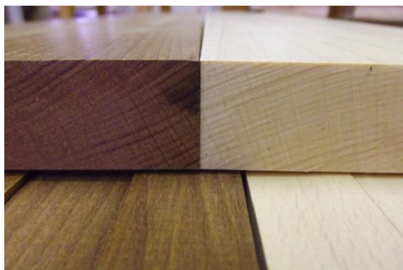
Fig. 2. Comparison of thermally modified beech wood (left) and unmodified beech (right)
