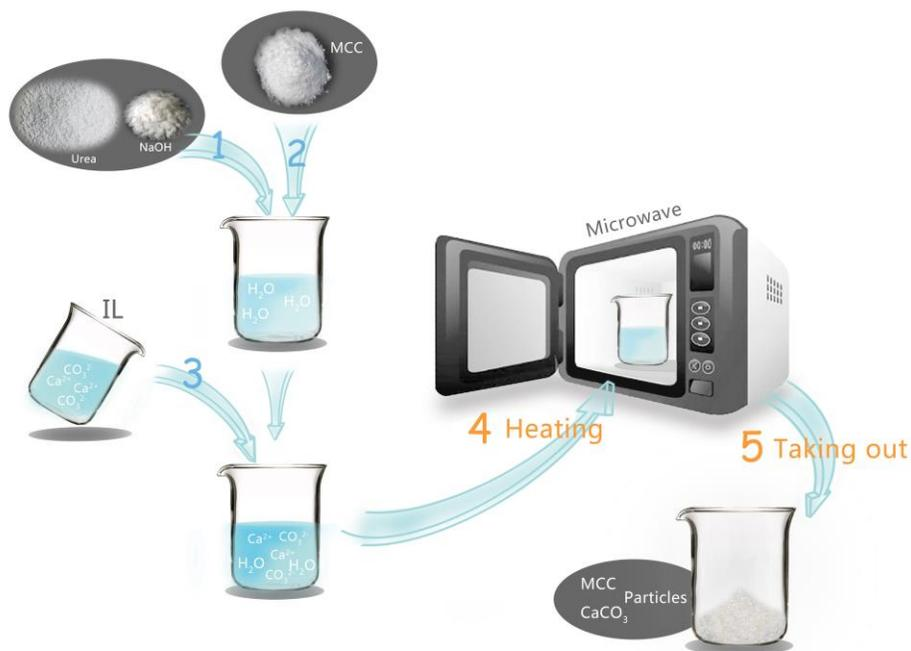
**Fig. 1.** Schematic image of the synthesis of cellulose@CaCO<sub>3</sub> composites using a microwave-assisted route
