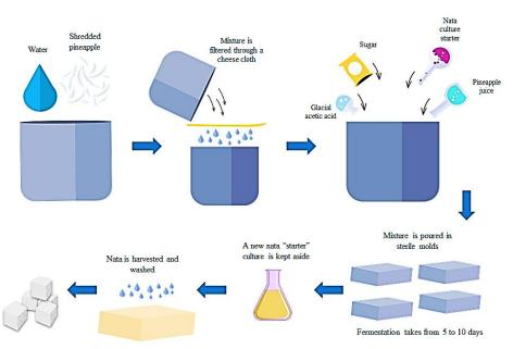
Fig. 5. Schematic representation of the Nata de pina production process
