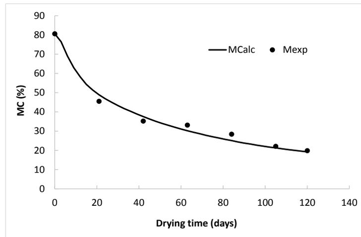
**Fig. 3.** A comparison between the experimental results ( $M_{exp}$ ) and calculated curve ( $M_{calc}$ ) using the software (Run1: from April to August, 2013)
