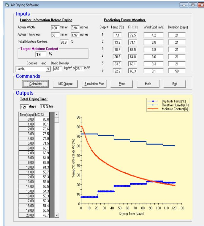
Fig. 2. User interface screen to estimate the air-drying rate (from April to August, 2013)
