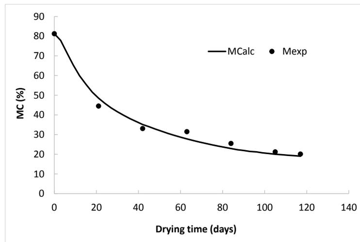
**Fig. 4.** A comparison between the experimental results ( $M_{exp}$ ) and calculated curve ( $M_{calc}$ ) using the software (Run 2: from July to October, 2013)
