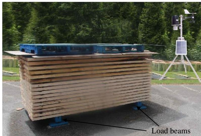
Fig. 1. Lumber stack, weather station, and load beams
