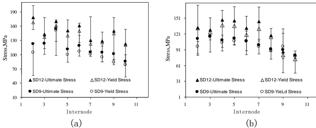
**Fig. 9.** Tensile strength of maize stalk rind of two varieties (SD12 and SD9) and moisture contents. (a) MC=80% (fresh) and (b) MC=8% (air dried)
