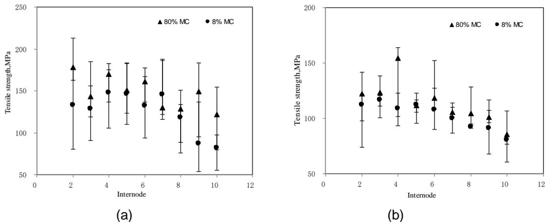
**Fig. 8.** Tensile strength of maize stalk rind at 80% (fresh) and 8% (air dried) moisture contents. (a) Variety SD12 and (b) Variety SD9.
