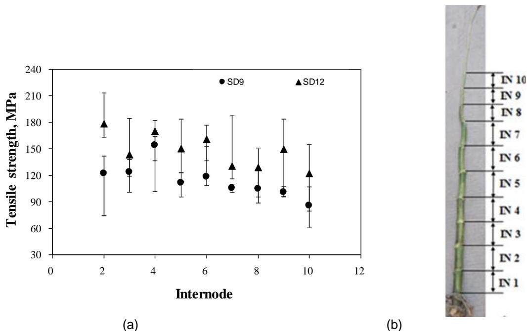
Fig. 7. Variation of tensile strength of maize stalk rind along the height at 80% moisture content (fresh stalk); (a) strength and (b) locations of internodes
