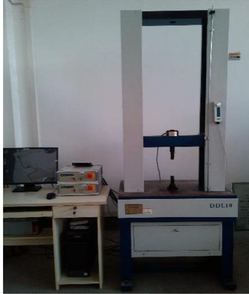
**Fig. 3.** Schematic diagram of the universal testing machine
