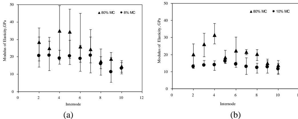
**Fig. 10.** Modulus of elasticity of maize stalk rind at 80% (fresh) and 8% (air dried) moisture contents. (a) Variety SD12 and (b) Variety SD9
