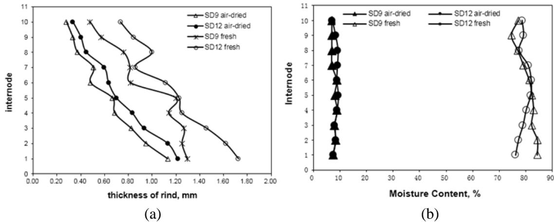
**Fig. 4.** Variation trend of the thickness of rind (a) and moisture content (b) for fresh and air-dried specimens
