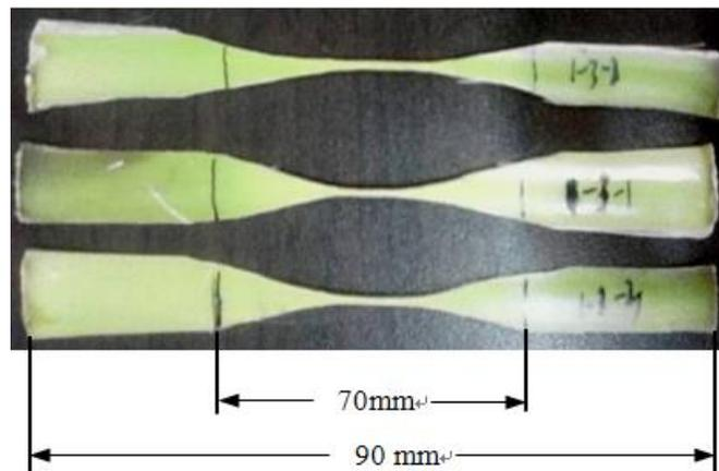
Fig. 2. Maize stalk rind specimens prepared for tensile test
