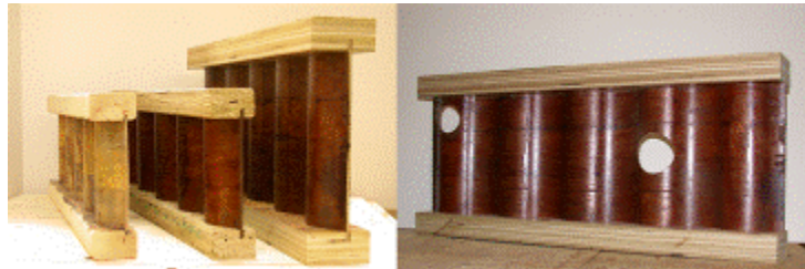
Fig. 1. Wood-based I-joists with 5 mm, corrugated, veneer-waste web elements
