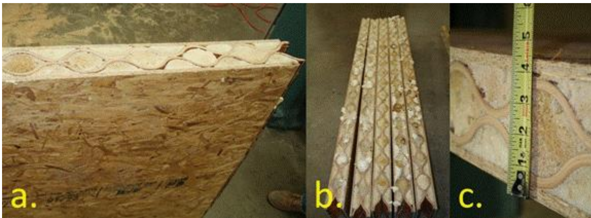
Fig. 9. Further use of corrugated panels. (a) SIP shear wall with PUR and corrugated panel core; (b) insulated beams for headers of building constructions; (c) one possible cross sectional configuration
