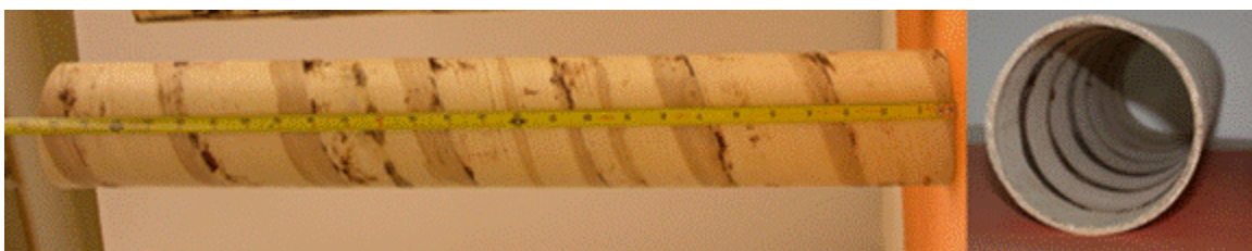
Fig. 10. Utilization of side clippings: 90-mm diameter tube for lightweight, pallet blocks
