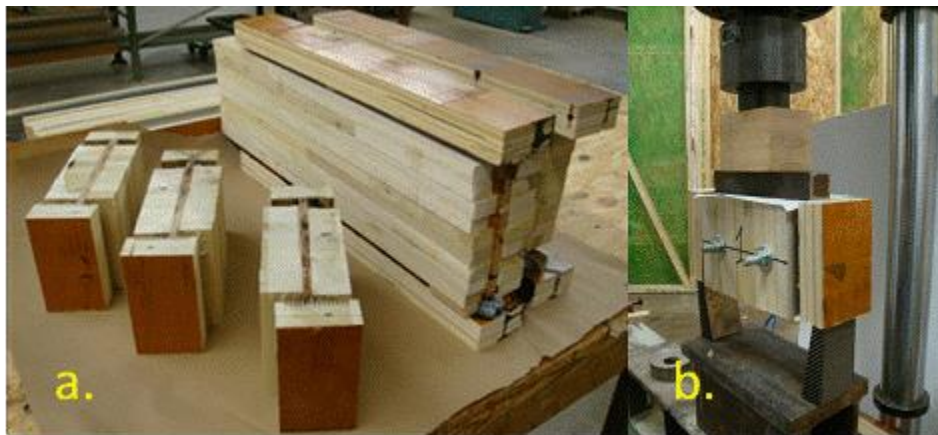
Fig. 6. (a) Preparation of specimens for web-to-flanges shear tests and (b) testing
