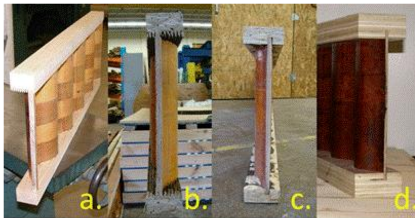
Fig. 3. Assembled I-joists with different flanges and joint configurations. (a) Spruce-pine-fir (SPF), finger jointed; (b) PSL, finger jointed; (c) LSL, grooved; (d) LVL, grooved
