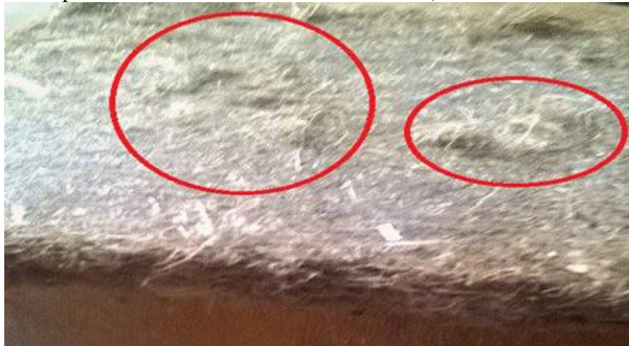
Fig. 2. The quality of hemp fibre boards at an assumed density of 300 \text{ kg/m}^3
