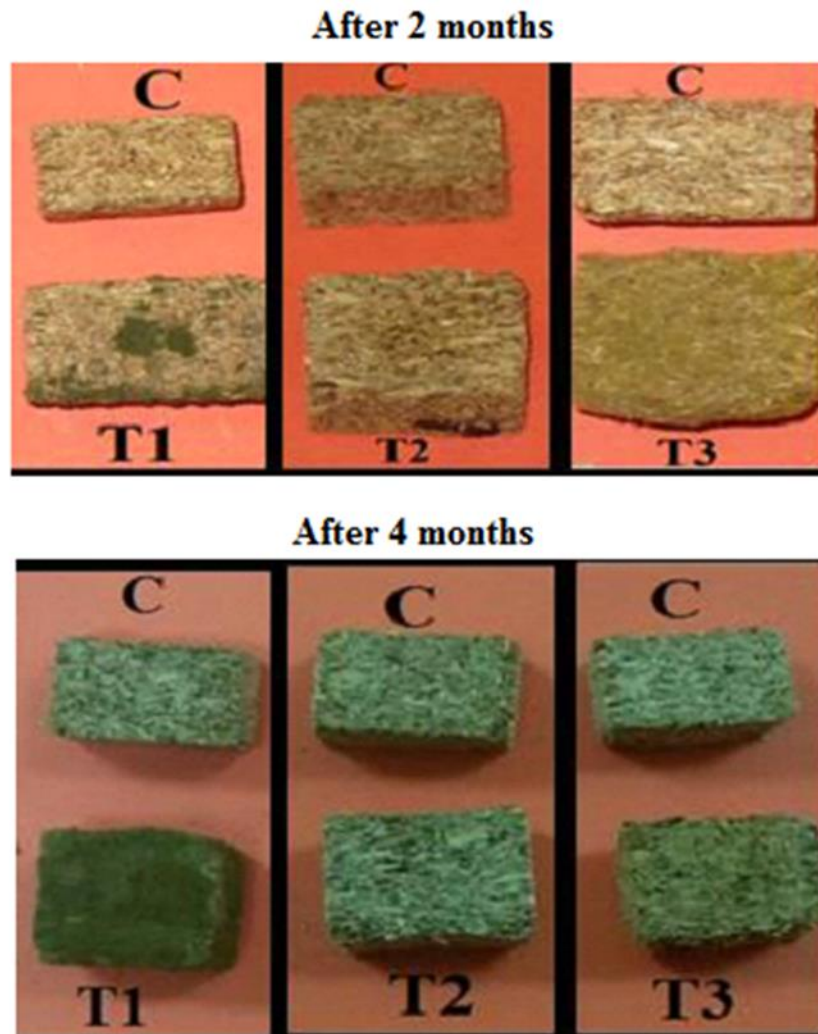
Fig. 4. Visual observation of the inoculated WPCs made from frond midrib of P. dactylifera wood by T. harzianum after 2 and 4 months
