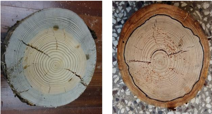
Fig. 9. Internal cracks inside red pine specimens after drying (left: control, right: PEG-treated)
