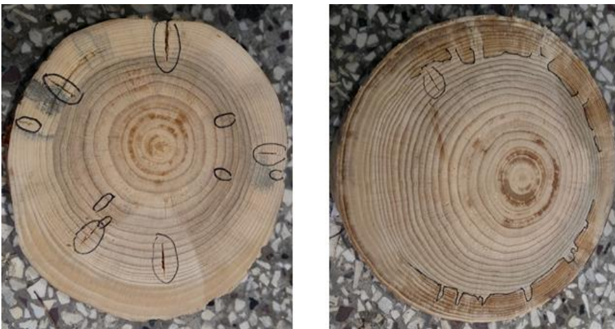
Fig. 10. Internal cracks inside Korean pine specimens after drying (left: control, right: PEG-treated)
