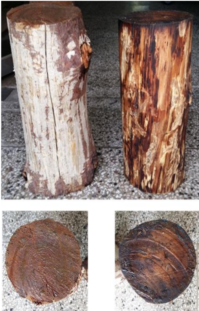
Fig. 8. Checks on surface layer and end surface of red pine round wood after drying (left: control, right: PEG-treated)
