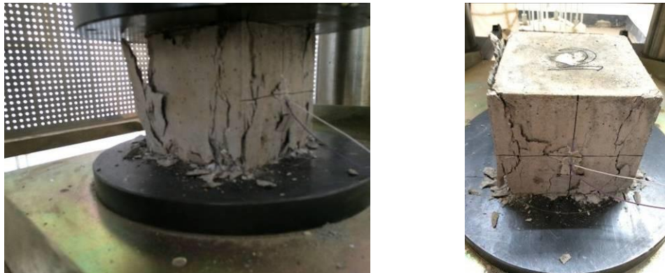
Fig. 3. Compressive strength tests of concrete
