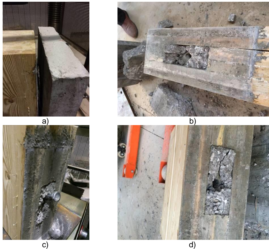
Fig. 7. Failure modes for timber-concrete composite specimens with stud-groove: a) timber is away from the concrete; b) cracks on timber; c) stud deformed and failed; and d) concrete failed
